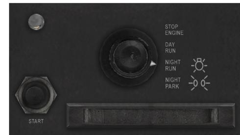
„Stop Engine“ shuts down the engine, release air pressure from doors and cuts all electric systems except the multiplex system.
