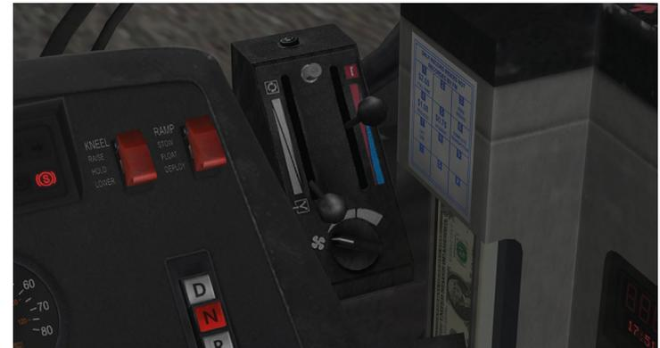
The console for driver's place air condition is placed in the middle of the windshield panel. Left lever is for blending fresh air and circulating air. Right lever is the temperature selector. The dial knob sets ventilation power for head and feet ventilation.
