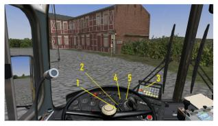
It's best to switch back to the driver view. You can turn on the onboard electrics by pressing [E] or by inserting the key (1) into the key switch and then pressing the main battery switch (2), which is directly above it. The IBIS startup chime will play and some of the warning lights and the IBIS display will light up (3). Note that some vehicles, like the '77 SD200 and SD202, don't have a battery switch. You'll only need to insert the key into the key switch to turn on the electrics.
